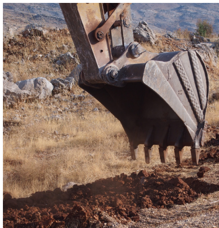
Figure 5-10. Excavator-prepared planting spot being refined with bucket dents
